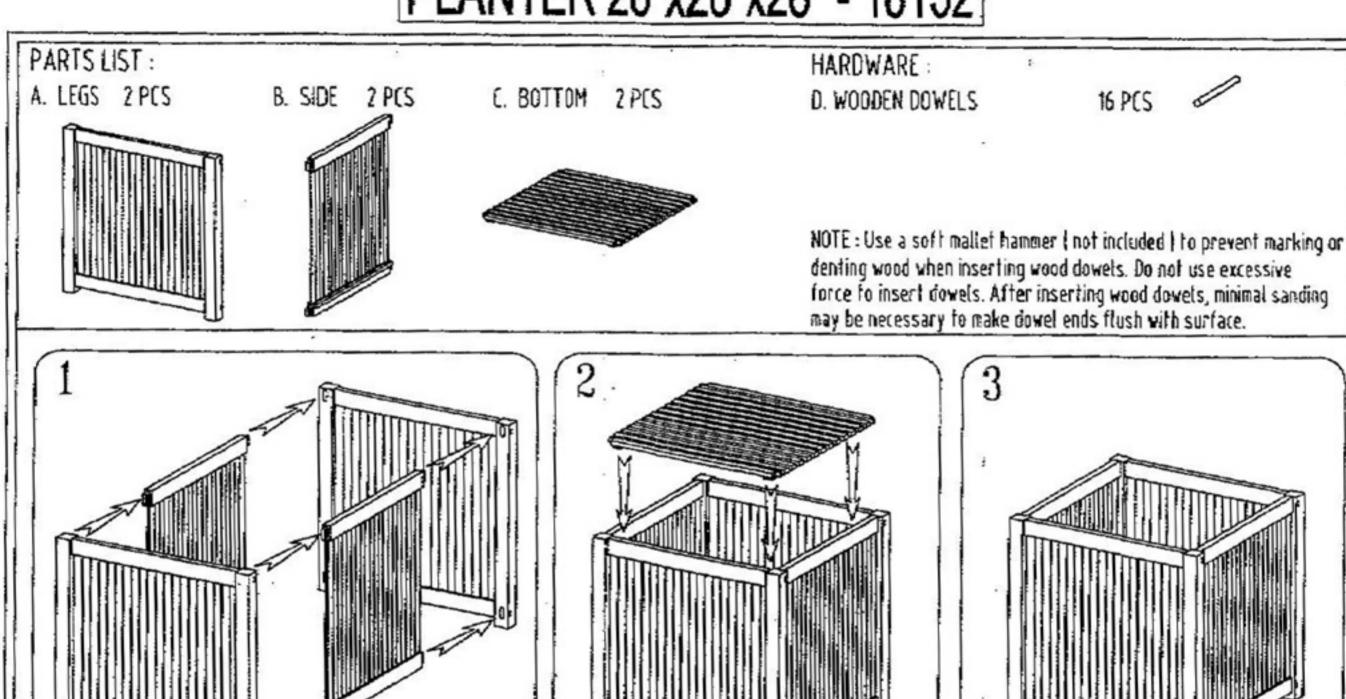
"IMPORTANT!! Each joint is unique, precise and will fit flush. You must match the white numbered labels with the corresponding number on opposite piece. Put all pieces together first to assure that all the joints fit flush then tap in the wooden dowels"
