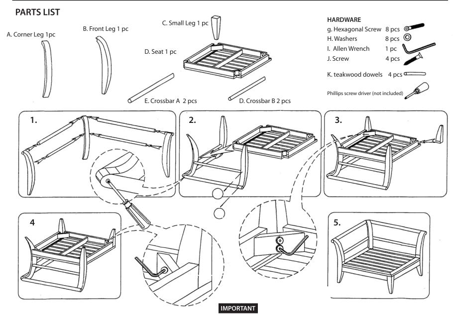
Each joint is unique, precise, and will fit flush. You must match the white numbered labels with the corresponding number on piece. Put all pieces together first to assure that all joints fit flush before tapping in the wooden dowels.
