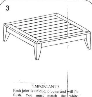
Each joint is unique, precise and will fit flush. You must match the white numbered labels with the corresponding number on opposite piece. Put all pieces together first to assure that all the joints fit flush then tap in the wooden dowels"
