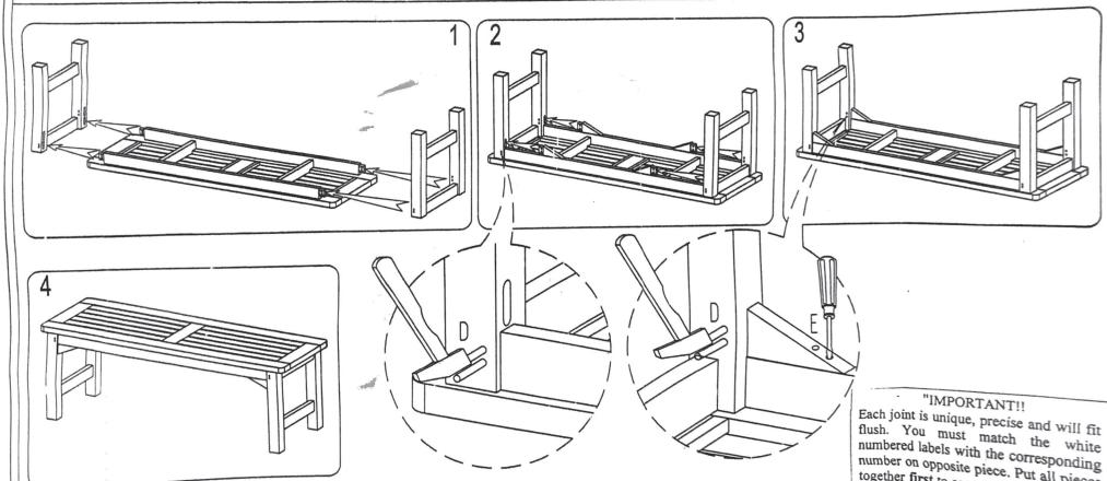
flush. You must match the white numbered labels with the corresponding number on opposite piece. Put all pieces together first to assure that all the joints fit flush then tap in the wooden dowels"
